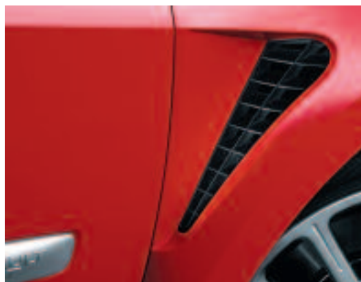
The extractor vents reduce turbulence.
